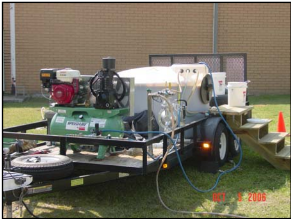
FIGURE 2. Mixing and injection equipment.
