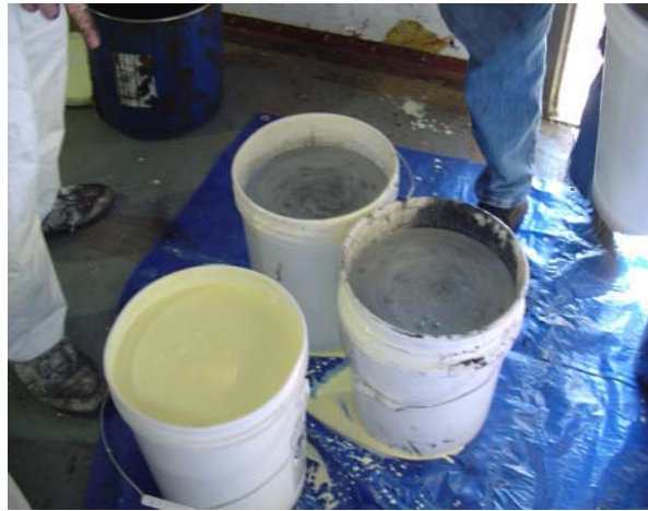
FIGURE 3. Concentrated emulsified vegetable oil amendment and zero-valent iron slurry.
